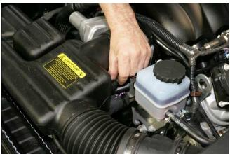
Loosen and remove screw clamp on throttle body.
