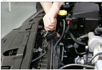
Using pliers, disconnect the wires connected to the lower support before removal.
