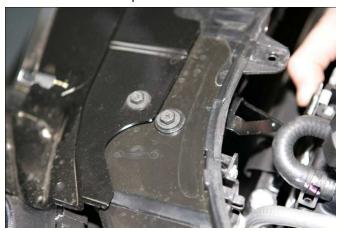
Using original 10mm bolts, holding A/C condenser onto radiator, screw the OTR radiator lean brackets into factory position. Now the bolt will go through the OTR bracket, the A/C condenser support, and into factory radiator bolt hole.
