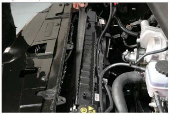
Place OTR in position, line up holes to factory locators
