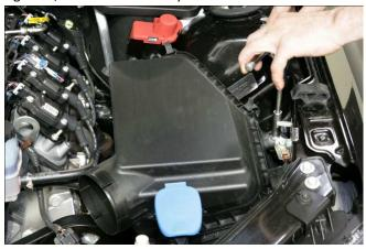
Insert flat head screwdriver into slot to raise radiator support bracket.
