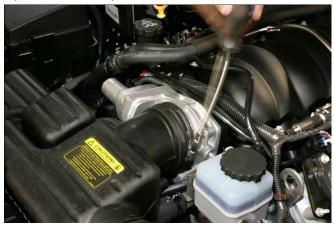
Loosen and remove screw clamp on MAF-meter - Airbox side, and disconnect from airbox.
