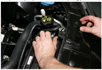
Tighten top bolts holding radiator 'lean' brackets in place.
