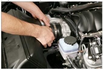
Use screw clamp to secure MAF coupling to throttle body. Again, for neatness, review the position of the screw clamp end.
