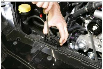
Loosen and remove 10mm bolt holding lower part of radiator support in place.
