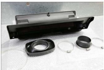
Fit MAF adaptor to MAF and tighten hose clamps, ensuring clamp is on the appropriate side.
