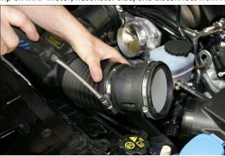
Loosen factory airbox grounding bolts, and remove factory airbox.
