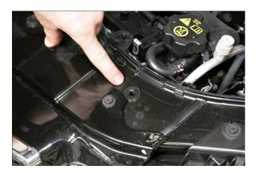
Use 10mm screw from lower radiator bracket for OTR brackets, on both sides. These brackets will lean the radiator for OTR fitment.
