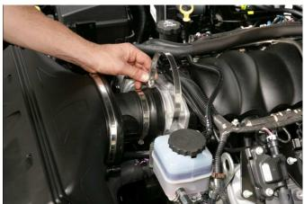
Using push clips provided, install into position along the front of the OTR, and press to secure. If not fully located, gently push side until clip pushes home.
