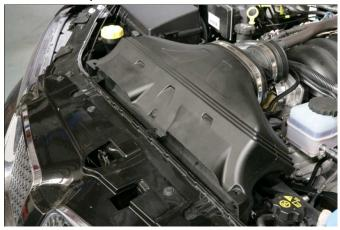
Gently slide the OTR into position, using the space provided by the new radiator supports.
