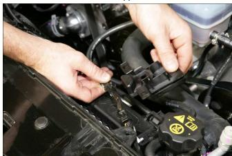
Remove 10mm bolt supporting A/C condenser
