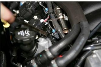
Using pliers, remove connector holding MAF wiring in place. This will assist the loom in reaching the MAF in its new position.
