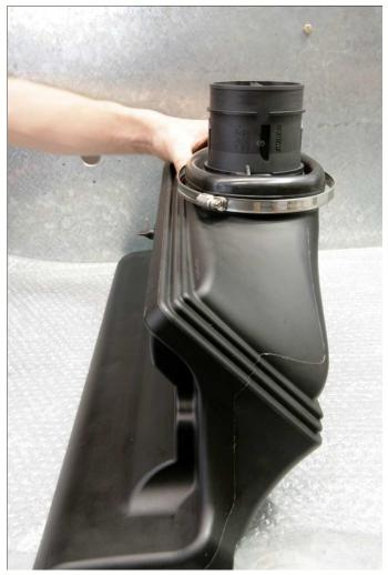
Shape and tighten the screw clamp to the OTR housing.
