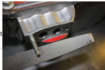
Figure 5 - Use a flat hand file to remove less than 1 mm of material until the spacer no longer interferes
