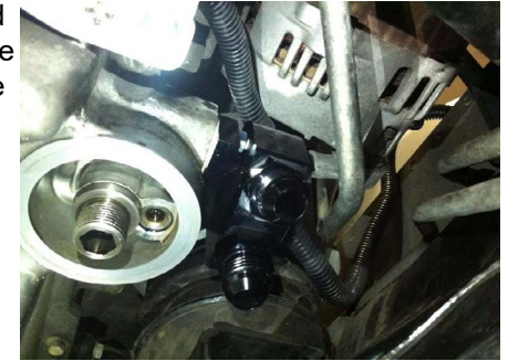
Figure 12 - Clearance gained between power steering line and oil cooler adapter
