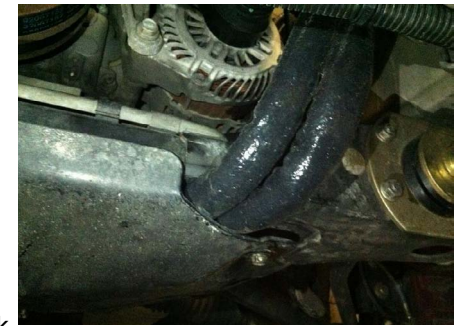
Figure 14 - Oil lines will run through the gap between the skid plate and front cradle
